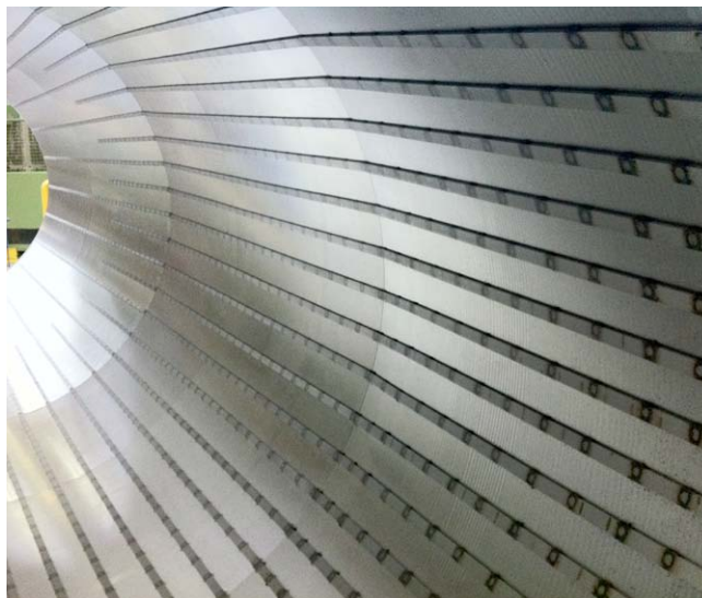
The inside of the bowl is fully protected against abrasive media.
